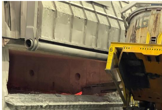
Figure 2. Metal pouring through MPTV.
